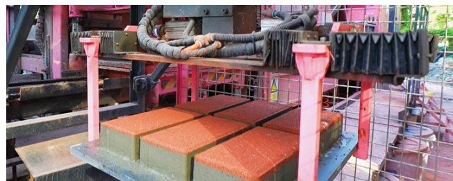
Colored pavement bricks produced by the mobile brick-making trucks
