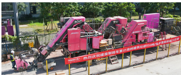
Mobile brick-making trucks for recycling construction waste
